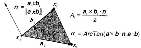
Fig. 2. Metric properties of the triangular tessellation.
