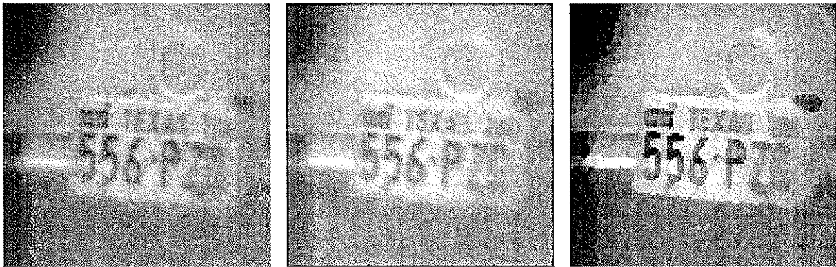
FIGURE 6.1. Subsampling with displacement vectors. Left: an image subsampled with bicubic interpolation. Right: the same image subsampled using the offset vector field.
